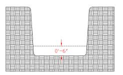
Excavate an area slightly larger than the outside demensions of the enclosure and 6 inches deeper to allow for a gravel base.
