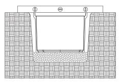
Fill the hole on the outside of the enclosure and compact as required.
