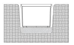
Carefully lower the enclosure into the hole and level the top with grade.
