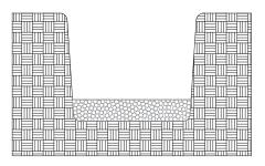
Add and level approximately 6" of gravel to the bottom of the hole.
